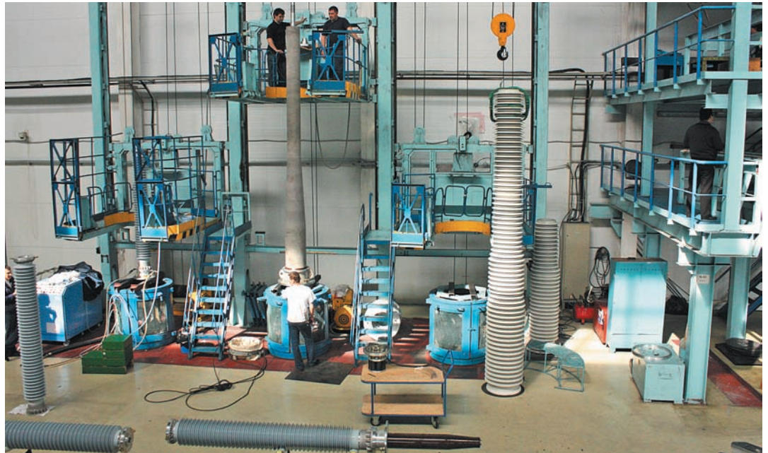
750 kV transformer bushing assembly at Izolyator
