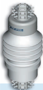
Removable Air – Oil bushings for power transformers Voltage: 20-35 kV Current: 6-20 kA
