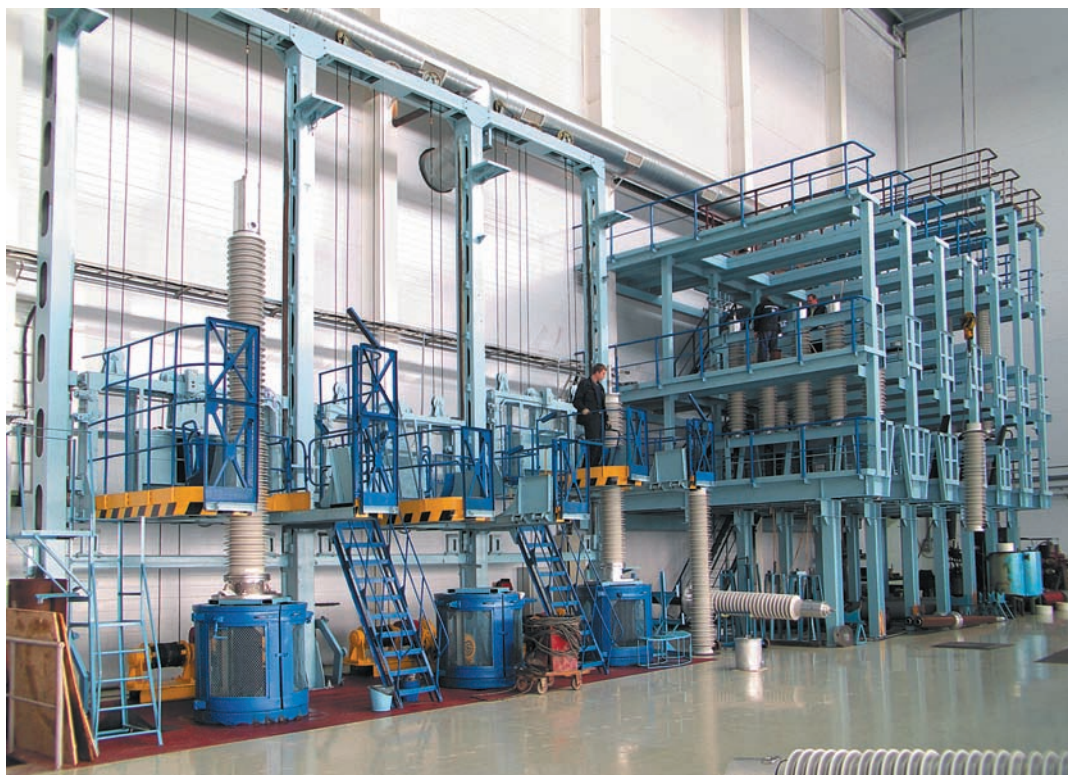
Assembly station of 220 – 1150 kV bushings
