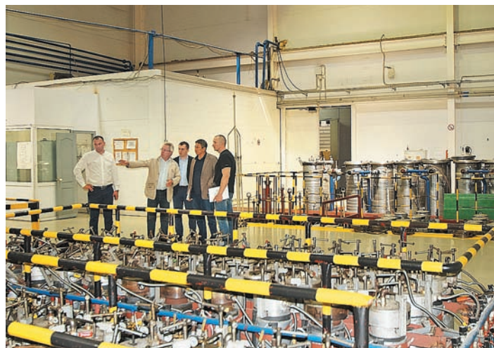
At the station of the internal insulation saturation and polymerization
