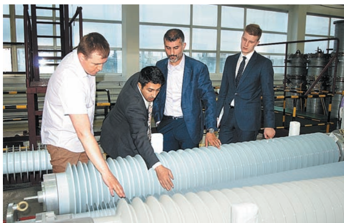
Side-by-side comparison of bushings by external insulation type
