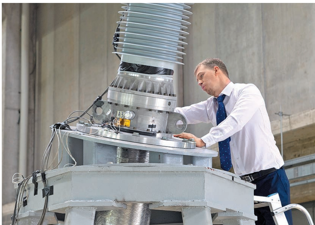
Deputy Chief Designer at Izolyator Pavel Kiryukhin checking the bushing's readiness for testing
