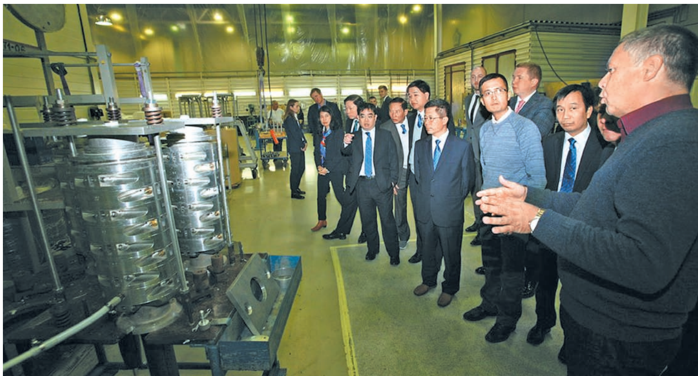
In the spotlight — casting moulds for external polymer insulation of bushings
