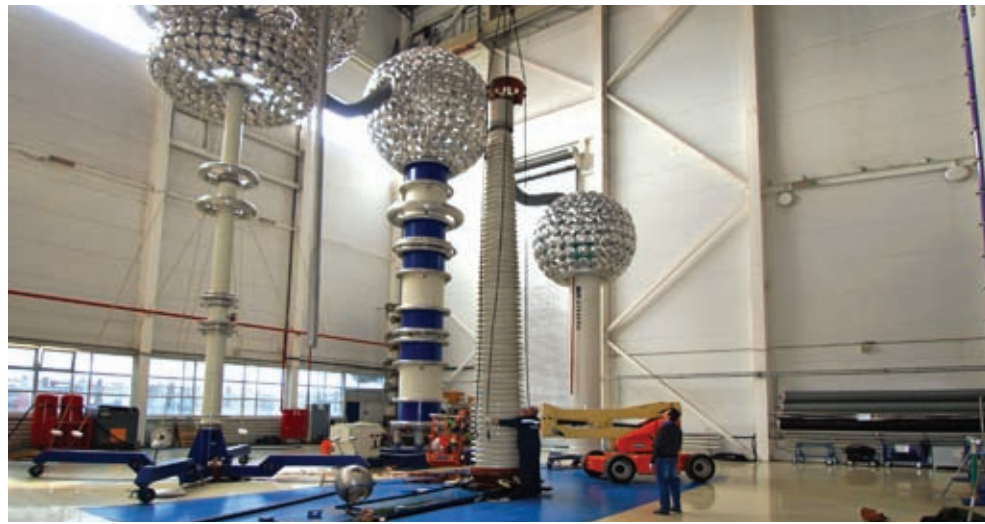
1150 kV bushing tests at Izolyator
