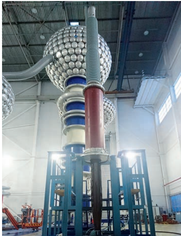
500 kV oil-SF6 bushing's tests at Izolyator plant
