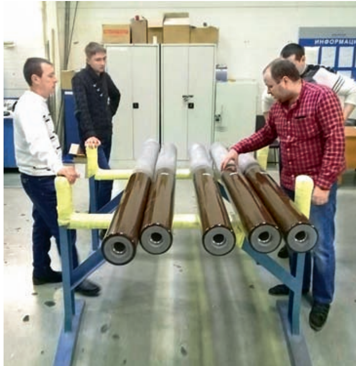
Kubanenergo specialists are learning about internal solid RIP insulation of high-voltage bushings production technology. Dmitry Mashinistov is giving the class
