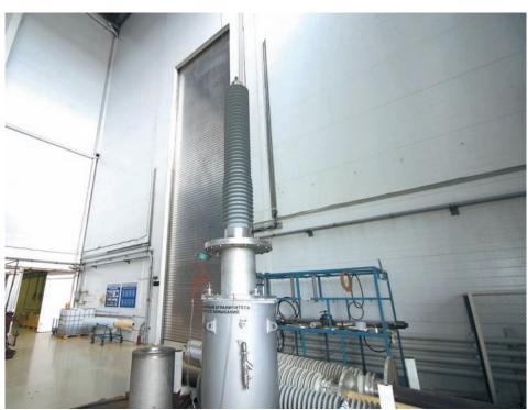
220 kV air-liquid nitrogen bushing tests at −200°C
