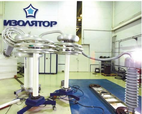
10-150 kV testing station of Izolyator's test center
