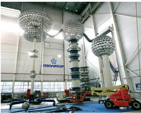
Series resonance test system of modular type for 1200 kV of alternating current
