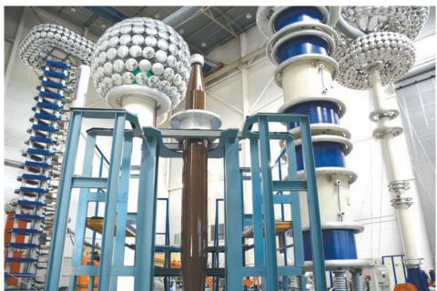
500 kV oil-SF6 gas bushing tests at Izolyator plant
