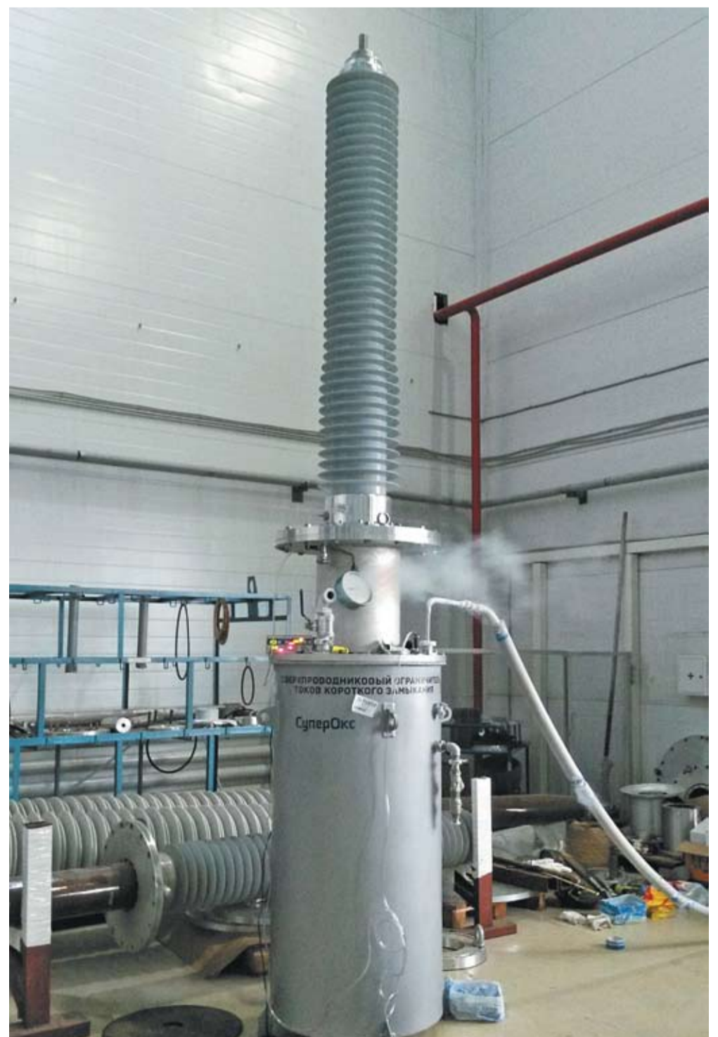
Fig.6 220 kV bushing in cryostat during the testing
