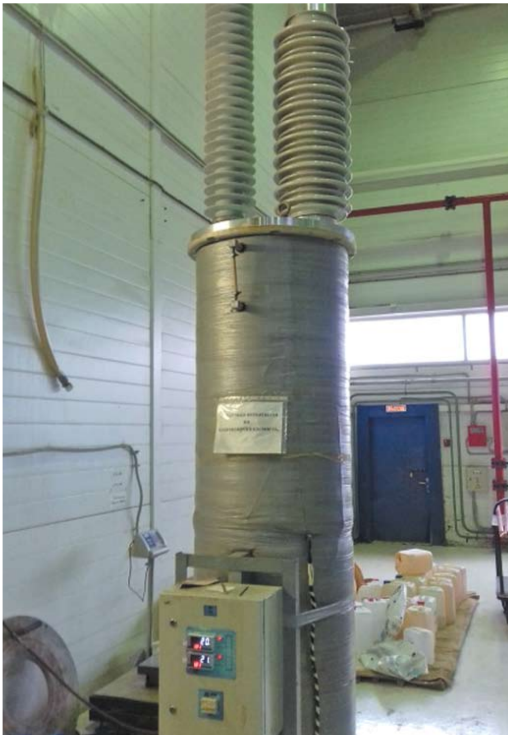
Fig.1 Test on moistening in a salt fog of 110 kV bushings
