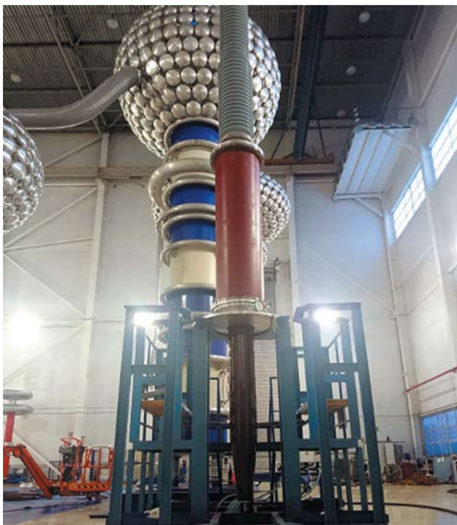
Tests of 500 kV Oil - SF6 gas bushing at Izolyator plant
