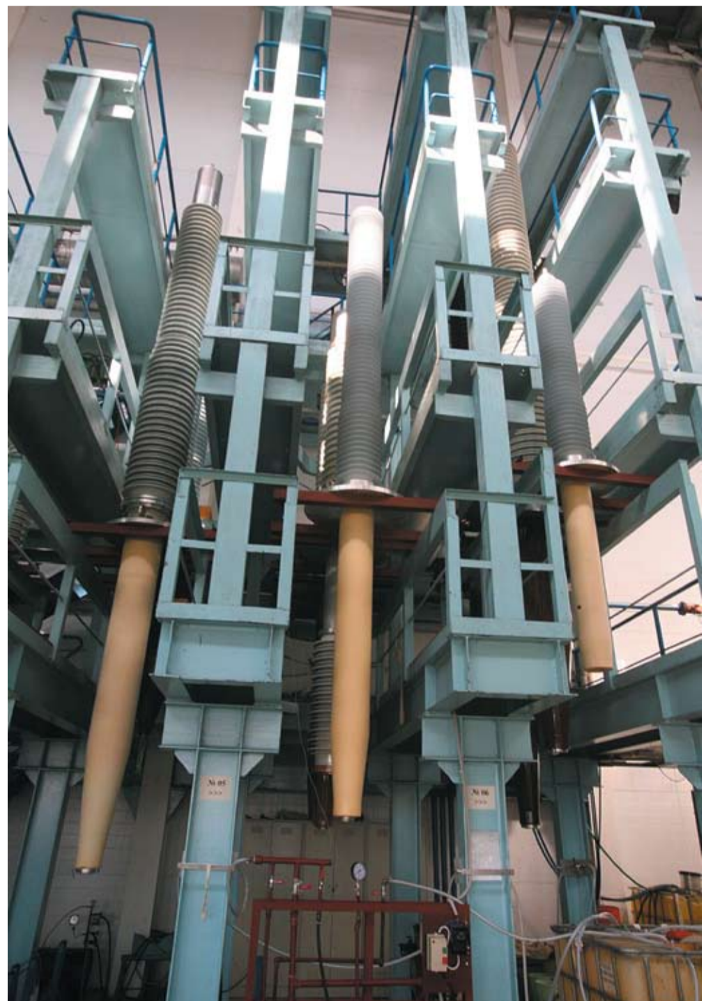
Fig.3 220-500 kV bushings at the assembly shop
