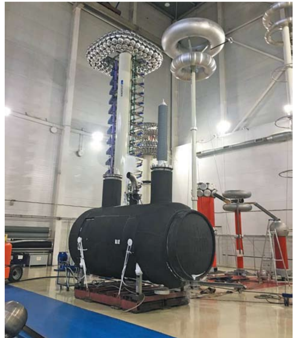
Current-limiting device of SuperOx design at the test center of Izolyator plant
