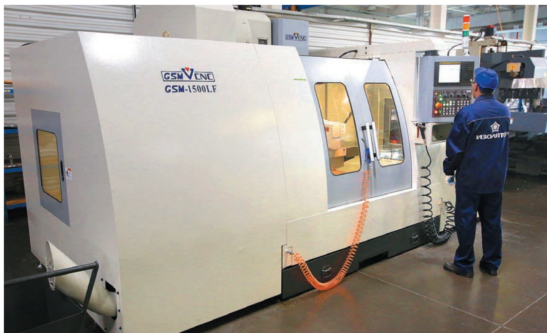
A new CNC milling machine at the mechanical shop of Izolyator plant
