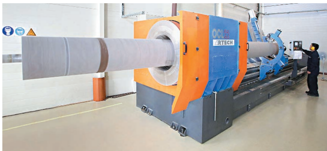
◀ The new machine for mechanical treatment of 500–750 kV insulation at the insulation making shop of Izolyator plant
