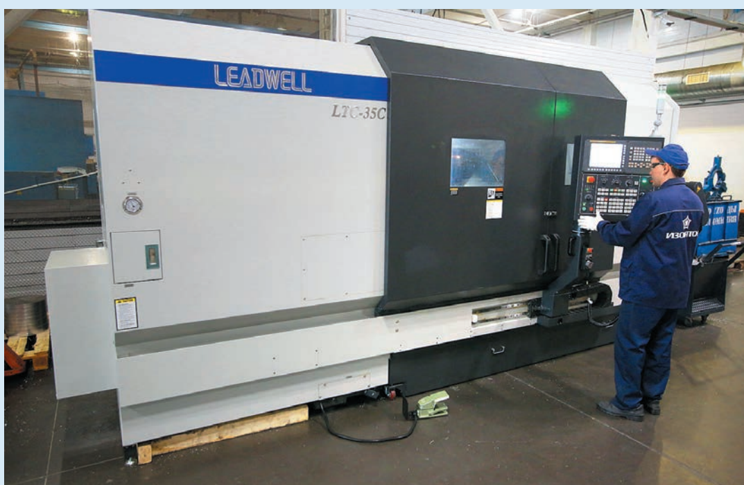
The New lathe machining center at the mechanical shop of Izolyator plant
