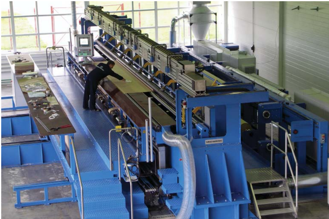
Fig. 1 High-production insulation winding machine 252–1200 kV
