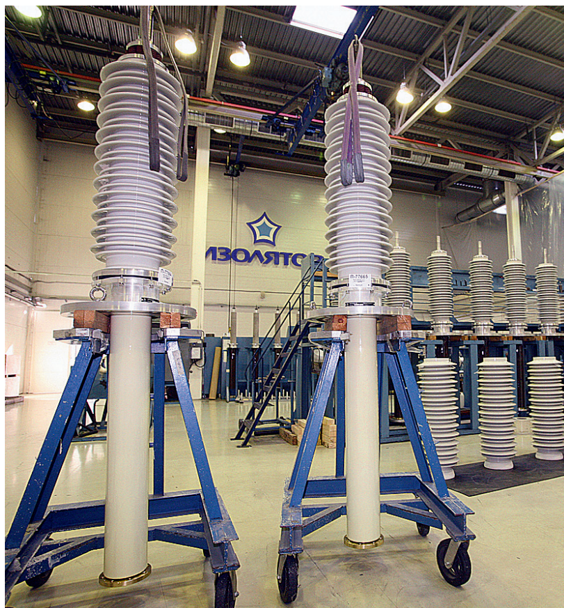
Assembly of RIN-insulated bushings for oil circuit breakers
