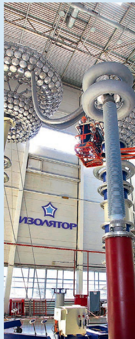
Testing of 500 kV Oil - SF6 gas bushings at Izolyator plant
