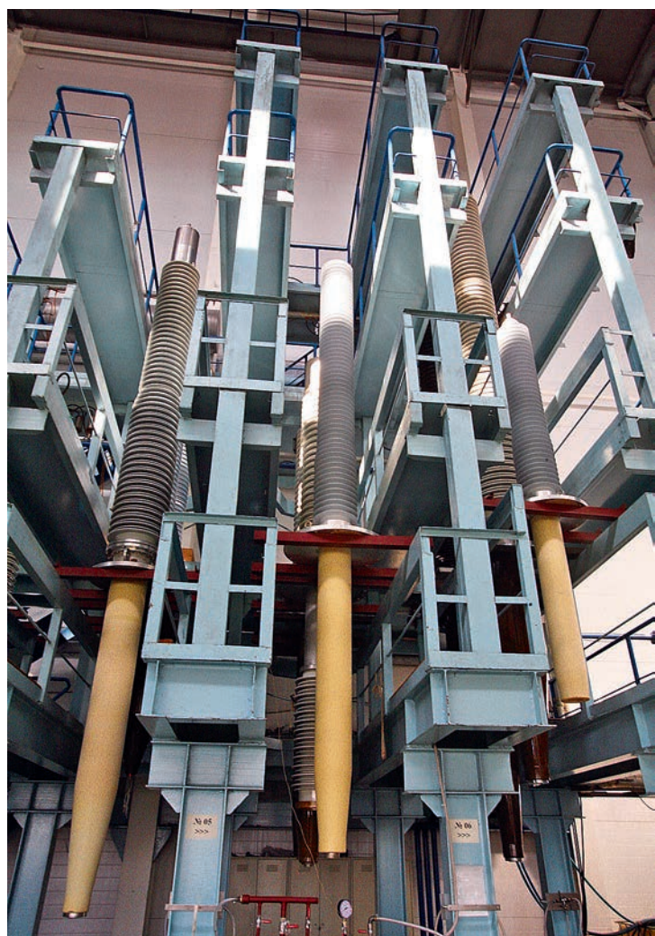
500, 330 and 220 kV RIN bushings placed on technological racks at the assembly shop of Izolyator Company
