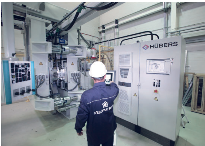
New equipment for manufacturing external polymer insulation of bushings at Izolyator plant
