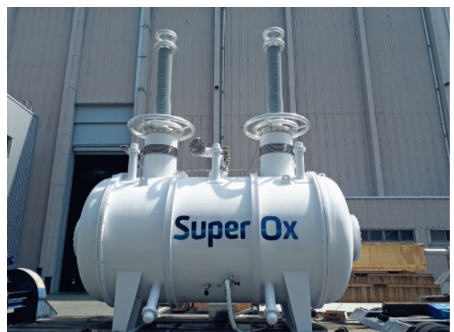
The first phase of 220 kV superconducting current limiter, equipped with bushings produced by Izolyator plant in the KER test center
