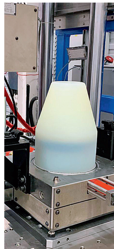
Stress cone for a 500 kV outdoor termination first time made in Russia at Izolyator-AKS plant
