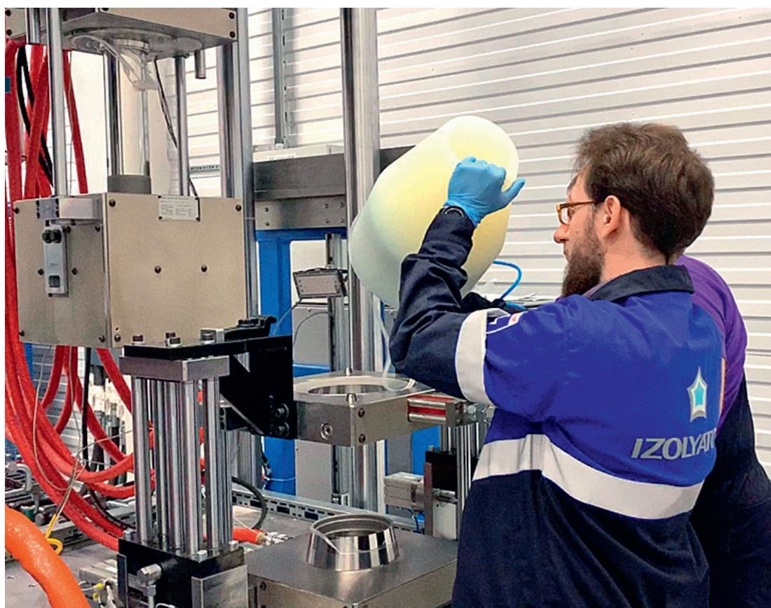
Stress cones production for terminating couplings at Izolyator-AKS plant
