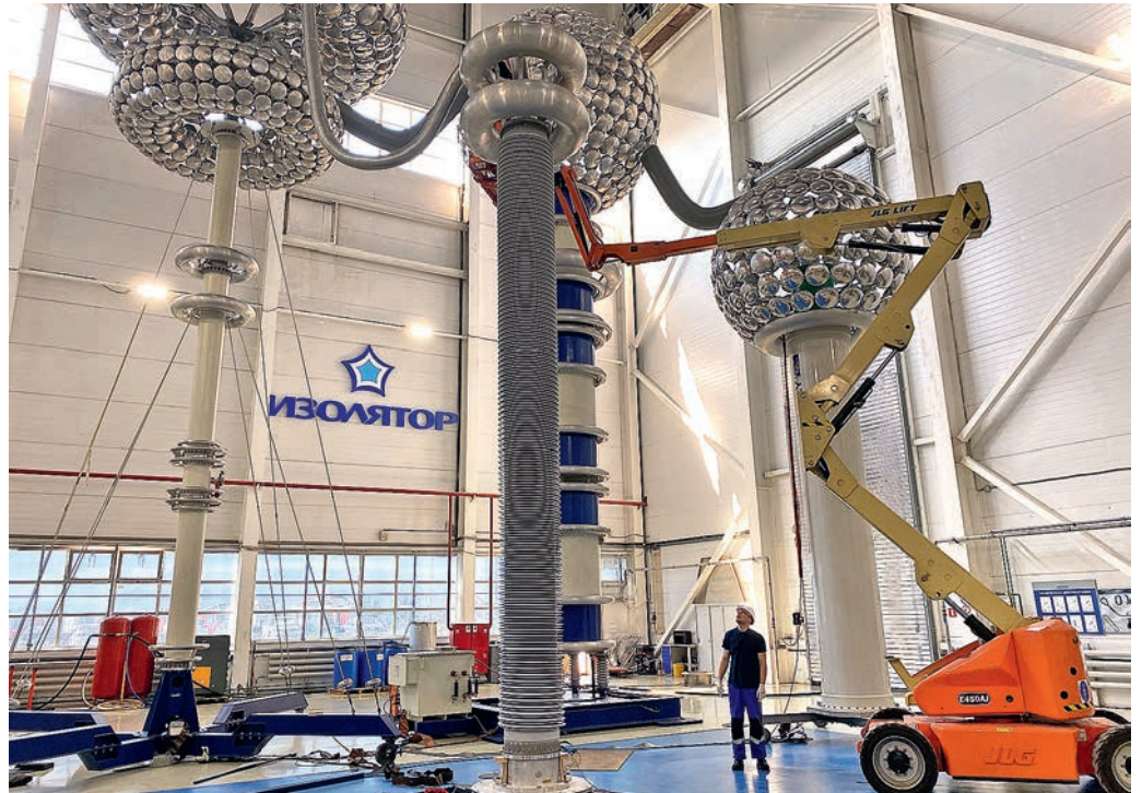
An Izolyator 800 kV / 2000 A bushing (C), made for the Indian state power grid company Power Grid Corporation of India Limited
