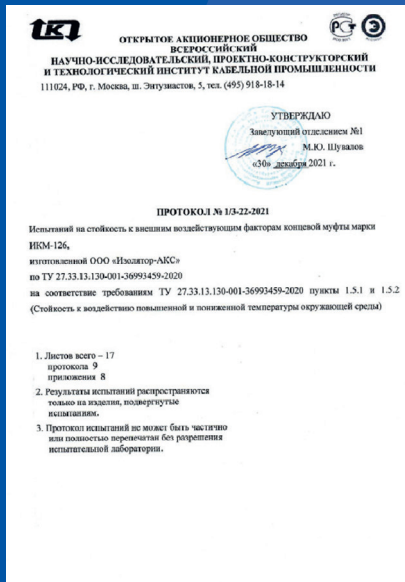
Tests for resistance to elevated and reduced temperatures from -60 to +50 °C
