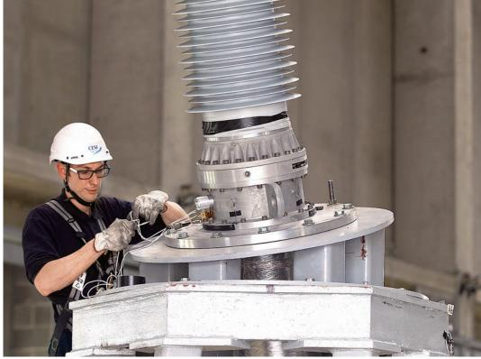
Installation of a bushing on a test rack
