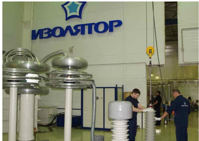
Fig. 25 Electrical tests of 126 kV bushings
