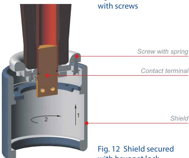
Fig. 12 Shield secured with bayonet lock
