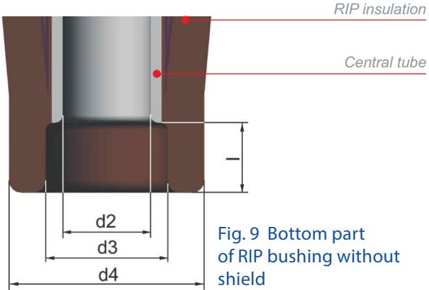
Fig. 9 Bottom part of RIP bushing without shield
