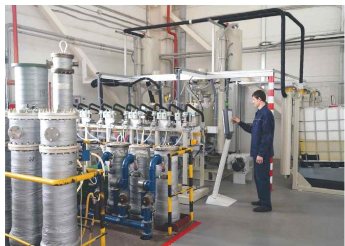
Fig. 19 Hubers machine for vacuum impregnation of insulation at Izolyator plant
