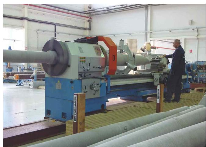
Fig. 20 Lathe turning of 550 kV RIP-insulation at Izolyator plant
