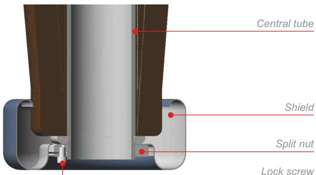
Fig. 11 Shield secured with screws
