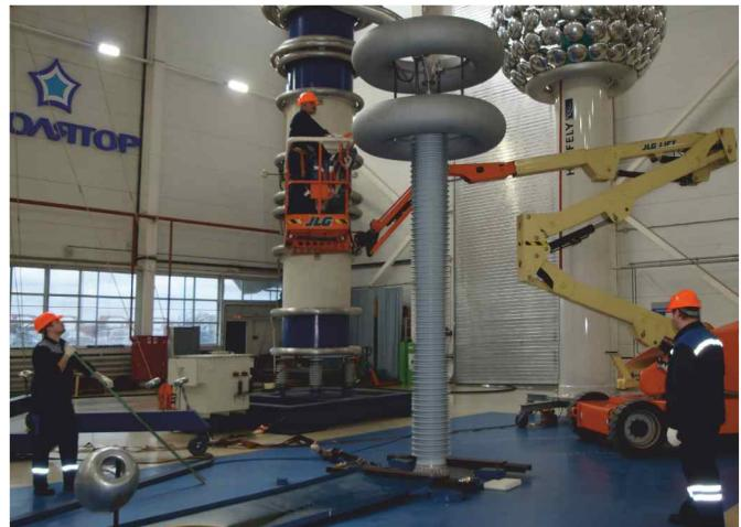
Fig. 24 252–1200 kV bushings test station
