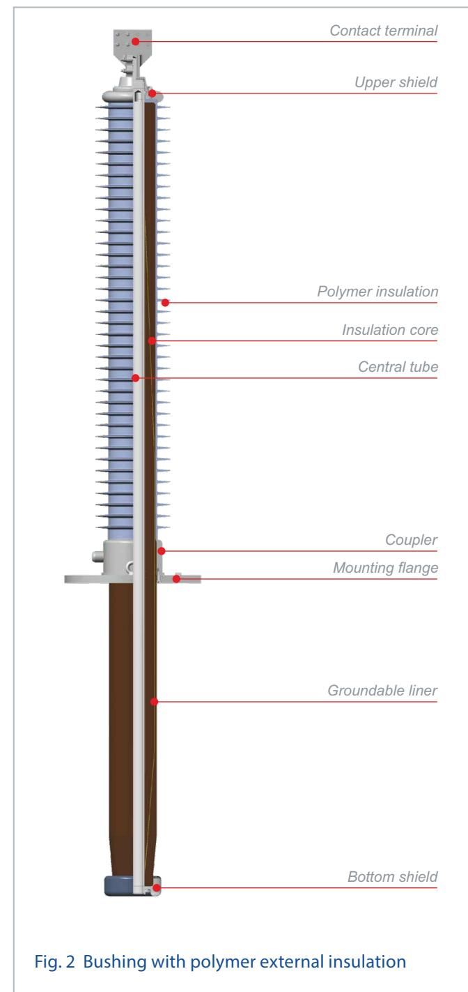
Fig. 2 Bushing with polymer external insulation
