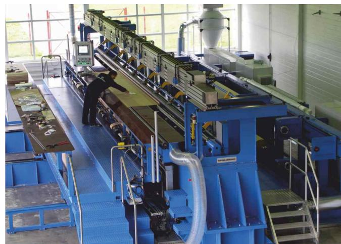
Fig. 18 Highly automated paper winding machine for 252 - 1200 kV bushings
