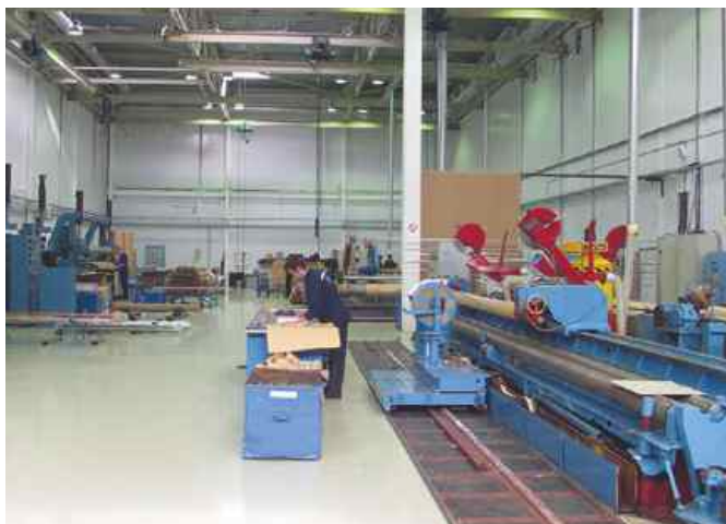
Fig. 8. Shop area of 40.5-800 kV paper insulation winding at the Izolyator plant
