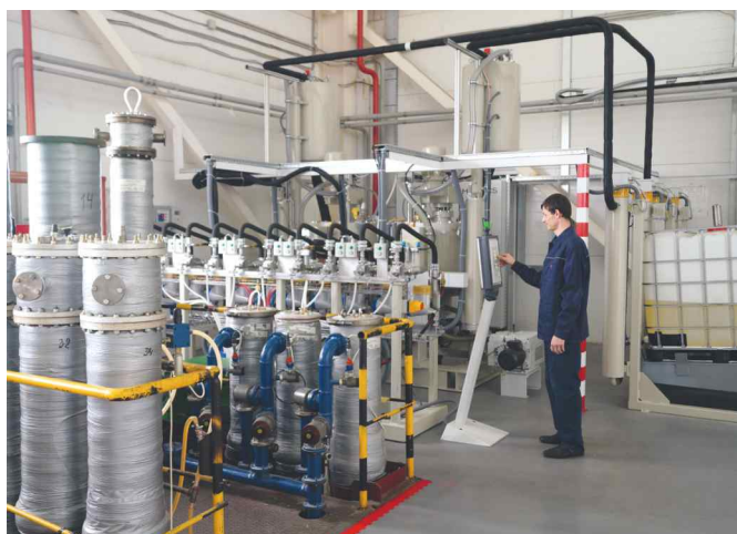
Fig. 9. Hubers machine for vacuum impregnation of insulation at the Izolyator plant
