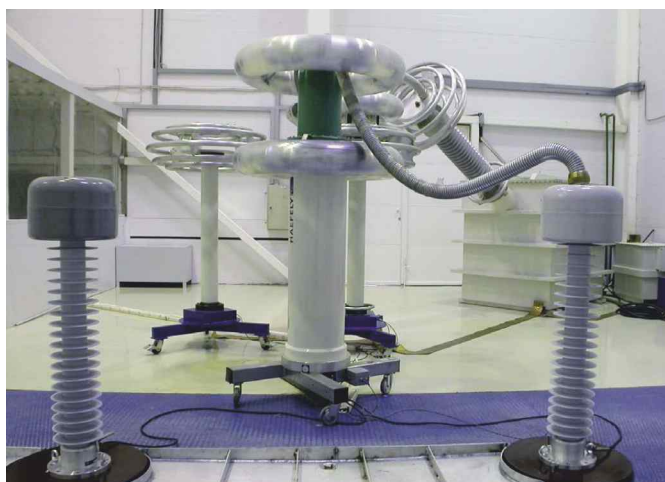
Fig. 15. Electrical tests of 126 kV bushings at the Izolyator plant
