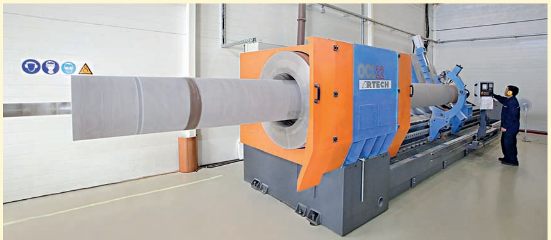
The new machine for mechanical treatment of 500 – 750 kV insulation at the insulation making shop of Izolyator plant
