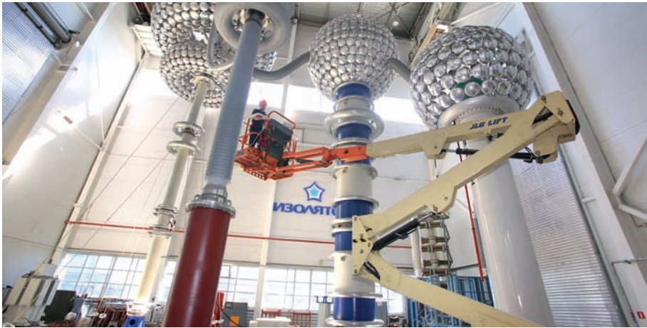
Tests of a 500 kV oil – SF6 bushing at Izolyator plant
