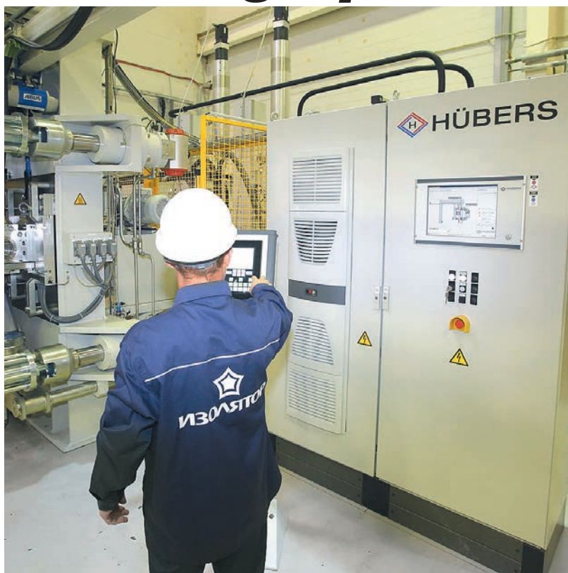
New Equipment for making of external polymer insulation of bushings at Izolyator plant
