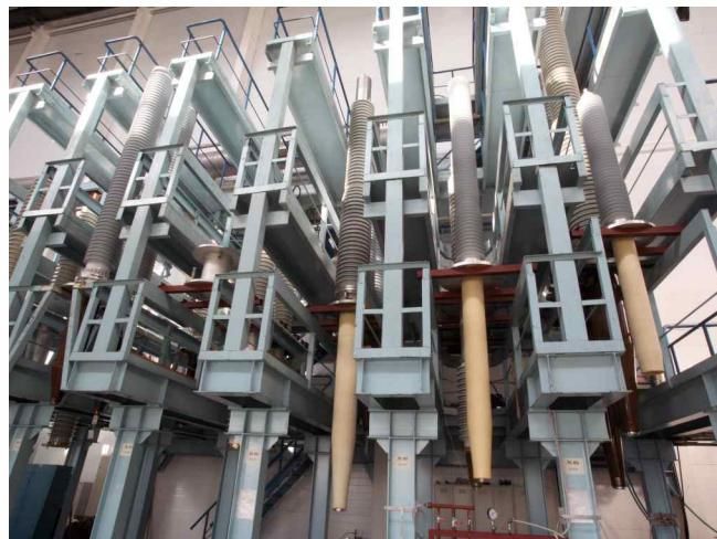
Fig.21 550, 363 and 126 kV bushings with RIN-insulation on technological racks at the assembly shop
