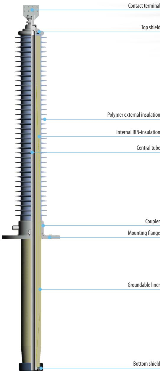
Fig. 2 Bushing with polymer external insulation
