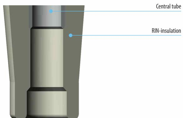
Fig. 9 Bottom part of a RIN bushing
