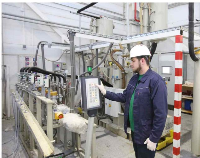
Fig. 19 Vacuum impregnation of main insulation
