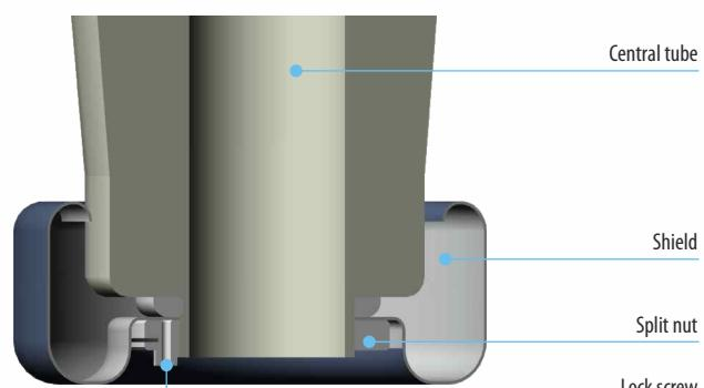
Fig.11 Shield secured with screws
