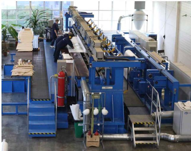
Fig. 18 Highly automated machine for winding the main insulation of 252 - 1200 kV bushings
