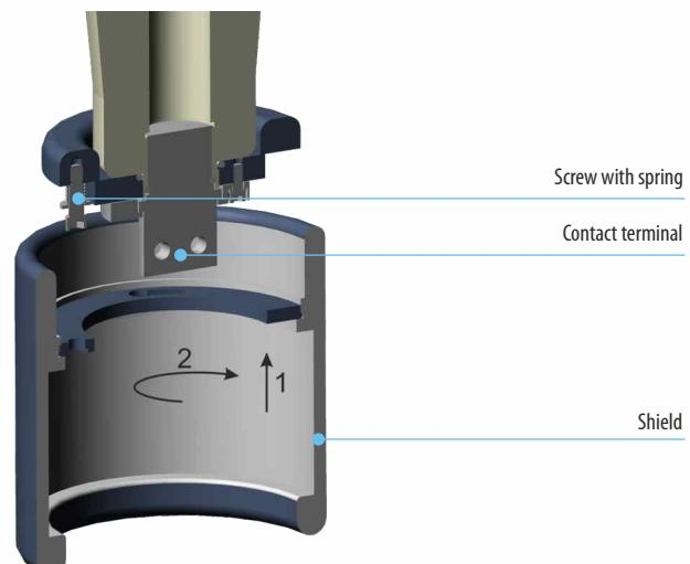
Fig.12 Shield secured with bayonet lock
