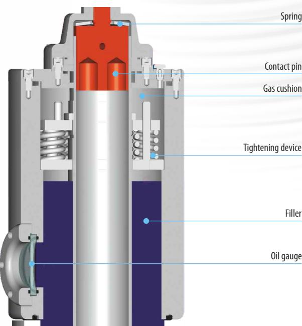
Fig. 6 Upper part of 252 kV bushings and higher with RIN-insulation and liquid filler
