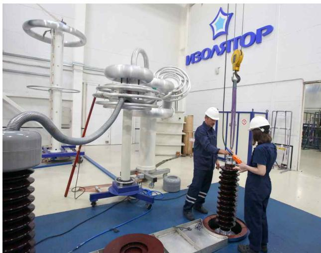
Fig.25 Electrical tests of 126 kV bushings
