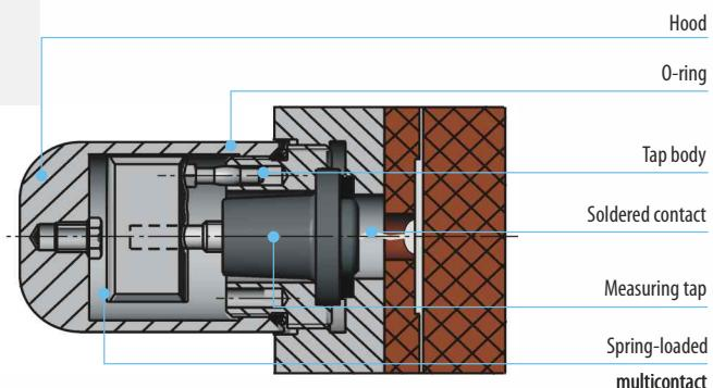
Fig.15 Measuring tap with grounded multicontact
