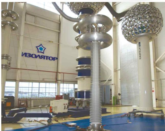
Fig.24 Electrical tests of a 550 kV RIN bushing at the test centre of Izolyator plant
