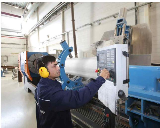
Fig. 20 Lathe turning of the insulation core
