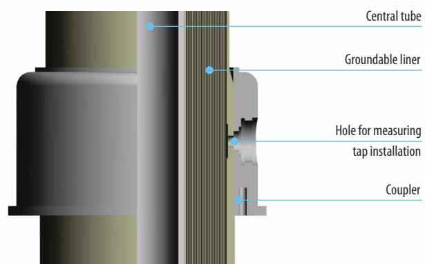
Fig. 3 Internal RIN-insulation
