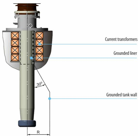
Fig.17 Installation diagram of current transformers
