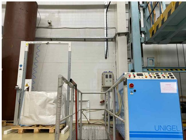
Fig.22 Unit for degassing and metering feed of compression gel
