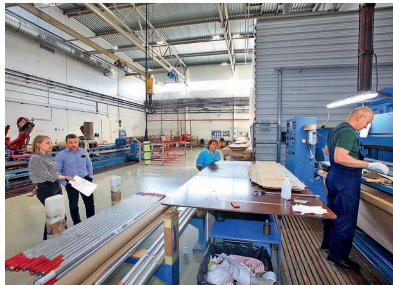
Checking the performance of qualifying work in the profession Winder of insulating core of the bushings
