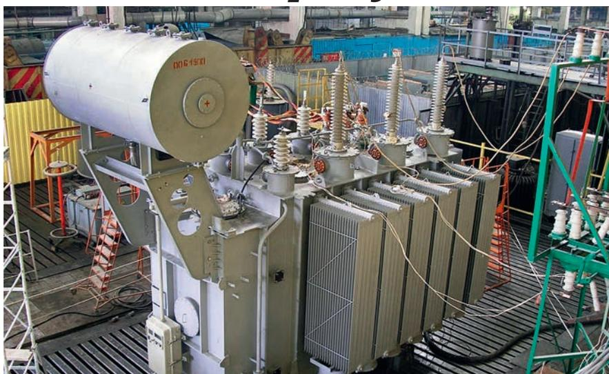
40 MVA 110 kV power transformer in the test center of the Togliatti Transformer plant (photo: Togliatti Transformer)
