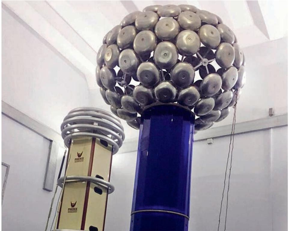
The state primary special standard of the unit of direct current electrical voltage, which has passed improvement - volt in the range of  $\pm (1 \dots 500)$  kV (photo: VNIIMS)
