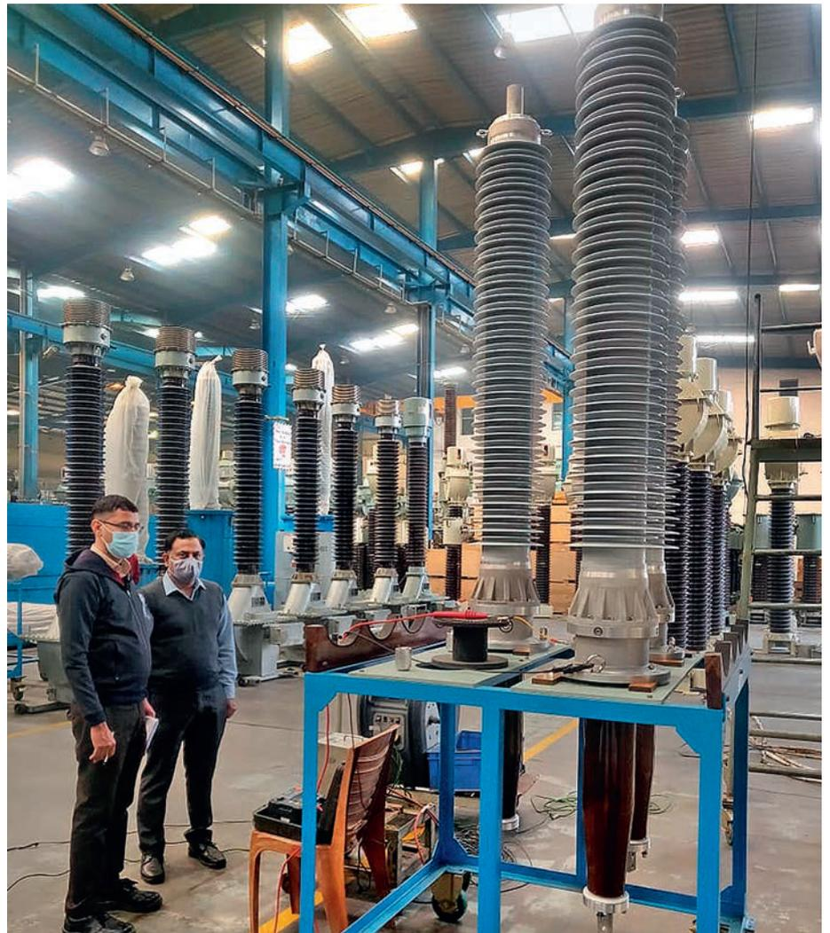
Inspection of manufactured bushings by the Power Grid Corporation of India Limited
