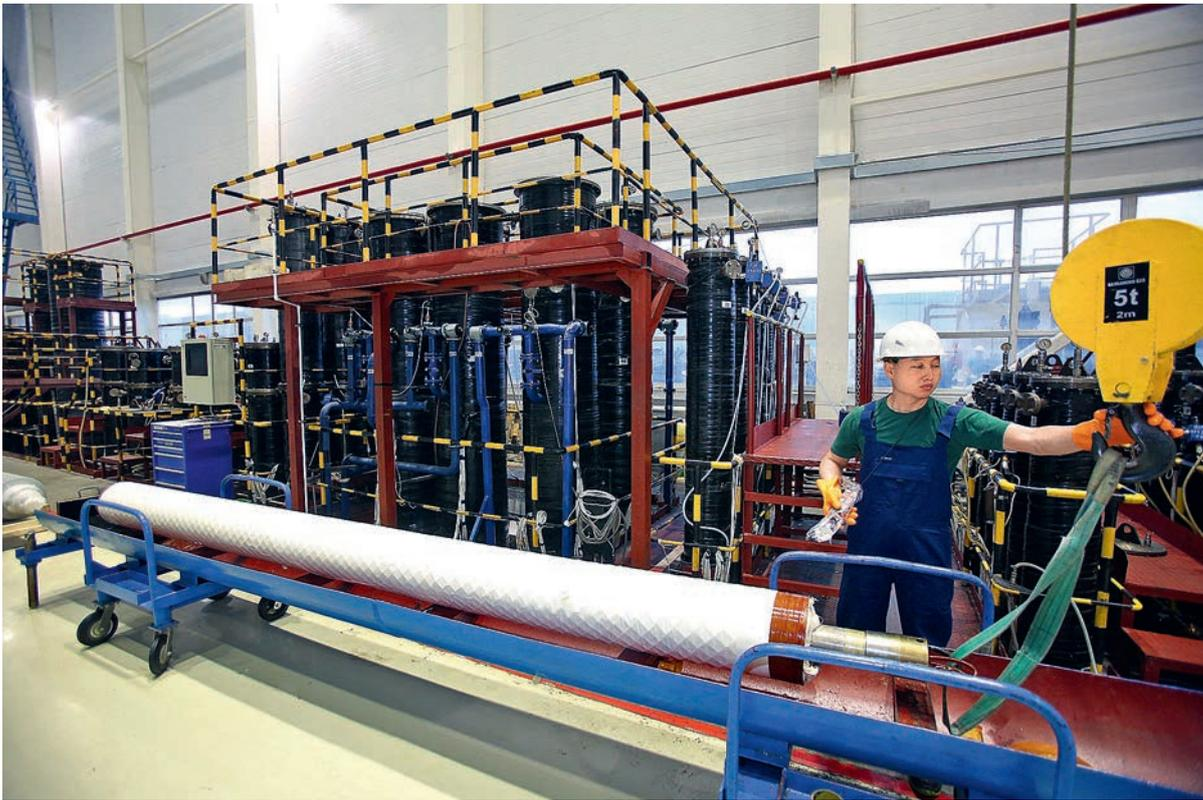
◀ The core impregnation - key process operation in the production of a bushing
