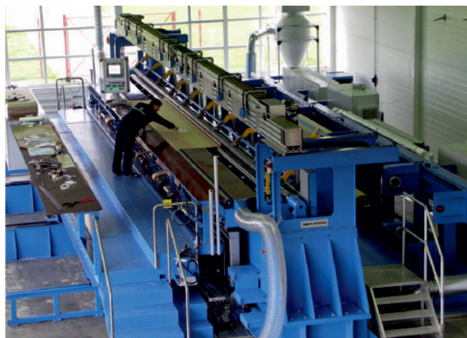
Fig. 18 Highly automated paper winding machine for 252 - 1200 kV bushings
