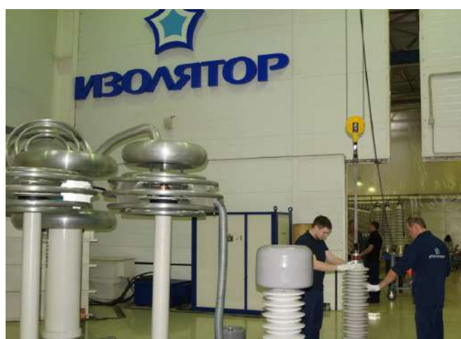
Fig. 25 Electrical tests of 126 kV bushings at Izolyator plant
