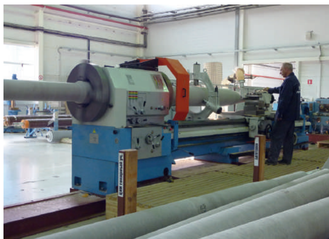
Fig. 20 Lathe turning of 550 kV RIP-insulation at Izolyator plant
