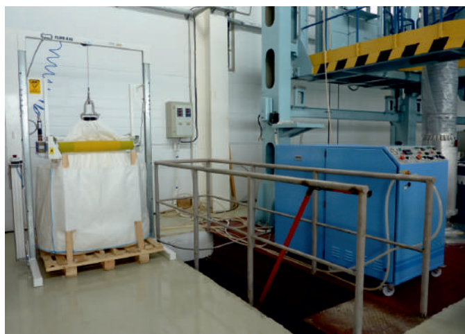
Fig. 22 Unit for degassing and metering feed of compression gel at Izolyator plant
