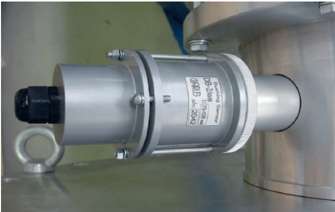
Fig. 16 Sensor for protection of the measuring tap
