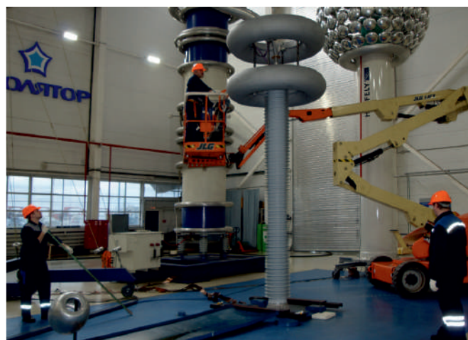
Fig. 24 252–1200 kV bushings test station at Izolyator plant
