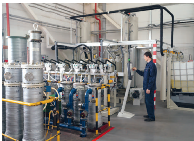
Fig. 19 Hubers machine for vacuum impregnation of insulation at Izolyator plant
